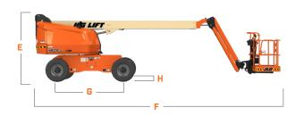
Platform Width 36-in / 0.91-m Platform Length 96-in / 2.44-m B. Machine Width C. 7-ft 6.8-in / 2.31-m D. Tailswing 2-ft 10-in / 86-cm E. Machine Height 8-ft 1-in / 2.47-m Machine Length F. 24-ft 11-in / 7.6-m Wheelbase G. 7-ft 9.5-in / 2.37-m Н. **Ground Clearance** 12.1-in / 31-cm
