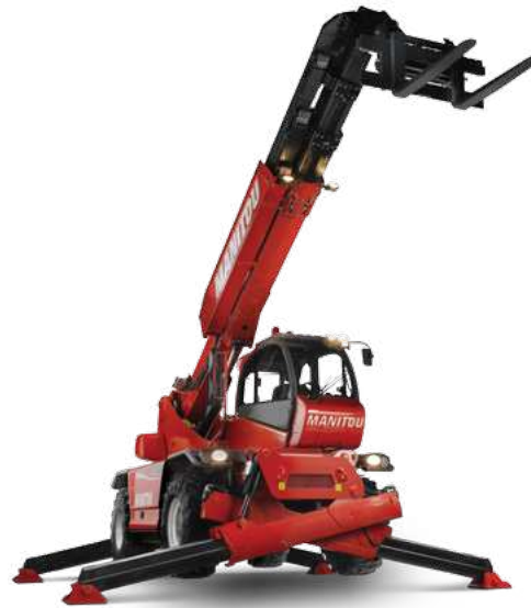
Rotation on lowered stabilizers with 1500 kg jib
