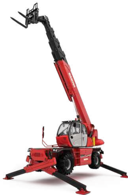
Rotation on lowered stabilizers with 1500 kg jib
