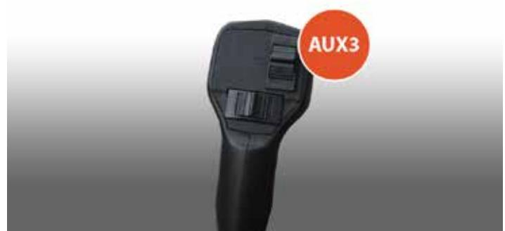
Proportional electronic roller for auxiliary hydraulic system
