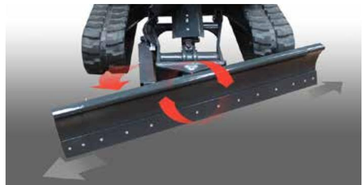
Hydraulic dozer tilt angle backfill blade with extension and
