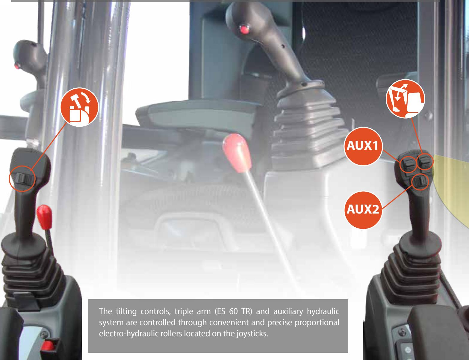
The tilting controls, triple arm (ES 60 TR) and auxiliary hydraulic system are controlled through convenient and precise proportional electro-hydraulic rollers located on the joysticks.
